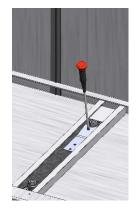
*Figure 15* – Bend Both Springs Back
