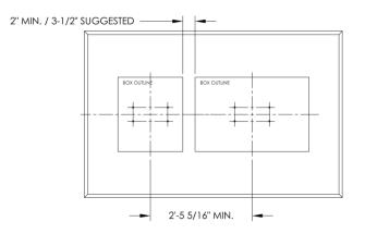
Figure 3 – versatile<sup>TM</sup> 4C Pedestal Single Column Unit Next to Double Column Unit
