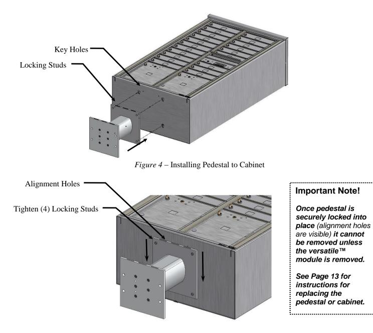
Figure 5 - Secure Pedestal to Cabinet by Setting Locking Studs
