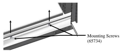
Figure 12 – Remove Bottom then Top Mounting Screws
